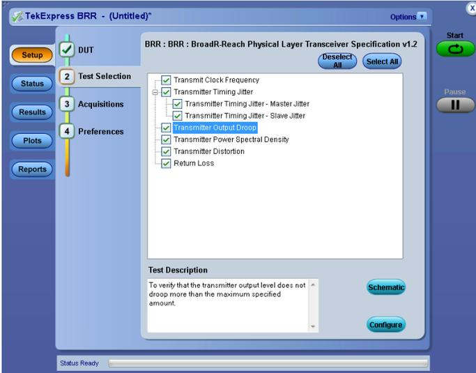
Tektronix Option BRR automates compliance measurements for BroadR-Reach 1.2 specifications. Option BRR simplifies test setup and eliminates human error resulting in more rapid compliance testing of BroadR-Reach designs along with reduced human error due to instrument setup. Engineers working on BroadR-Reach can turn to Tektronix for their complete PHY testing solution needs including fixtures.
